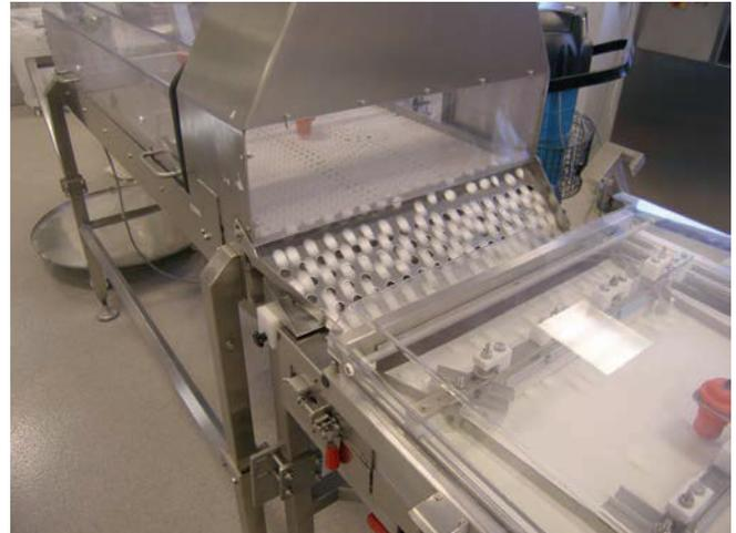
You need to have a fan to blow the air through the AirSlide®, the speed of the fan must be adjustable so you can find an air flow when the tablets is floating correct.
